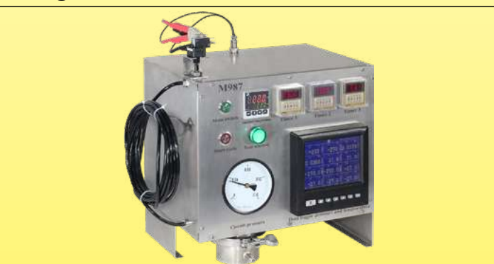
Test equipment for measuring repeatedly and constantly the maximum length of the air switch connecting tubes according to the volume of the push button and the pressure it develops (Ultimheat Laboratory)
